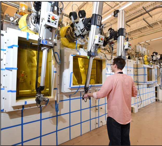
IMCL Shift Supervisor Jeffrey Bailey demonstrates manipulators on the hot cell side. The blue tape was used to map radiation levels, and will be removed for normal operations.
